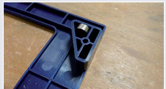
Afb. 6 Close-up magneet in Scharniermal
